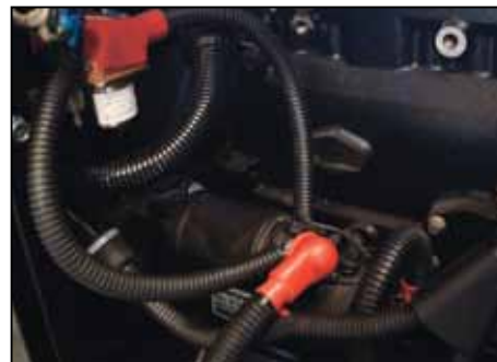
AC All wiring looms are encased in conduit with rubber boots fitted to avoid mechanical wear and damage.
